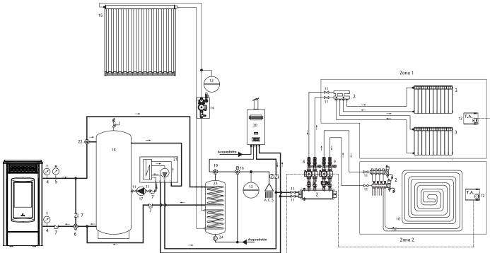
The diagram shown here is indicative and may not display all the components required to properly operate the system. Rely on a qualified thermal technician for the hydraulic system design.
