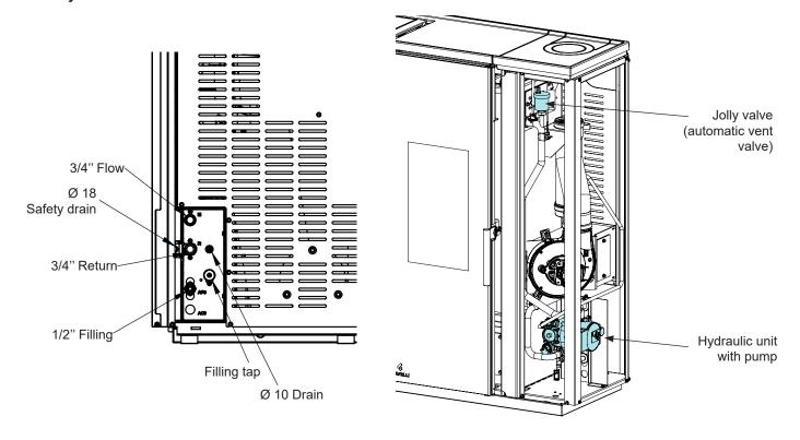
Connect the stove to the hydraulic system so as not to constrain it excessively and to allow it to move slightly.
