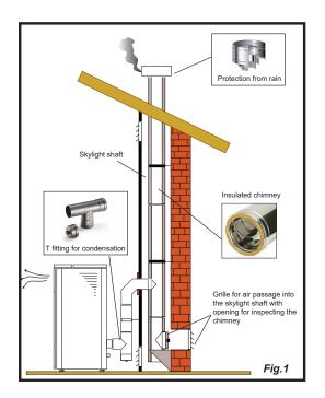
This type of installation (See Fig.1) requires an insulated chimney pot, even if the entire conduit is installed inside the building. Besides, the structure must be inserted into a properly ventilated skylight shaft.
